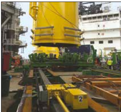
▼ The trolley system speeds up offshore wind transition piece load out: the transition pieces are positioned in the clamping frames and moved along the track.
